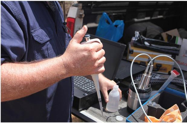
**Fig. 7** Precise calibration of the stream water with NaCl of a predefined concentration ( $10 \text{ g L}^{-1}$ )
