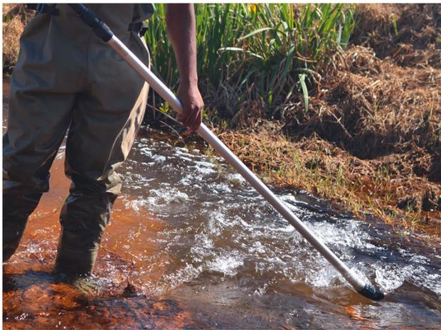
**Fig. 5** Flow measurement with an impeller meter at the Tweelopspruit (location N14) by the 2014 standard method of the CGS. Note that the impeller is placed incorrectly just below the water’s surface. The water is flowing from right to left, meaning that the operator is not within the reach of disturbing the flow measurement
