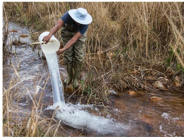
**Fig. 3** Slug injection of the NaCl solution at sampling location TFS (courtesy H. Coetzee)
