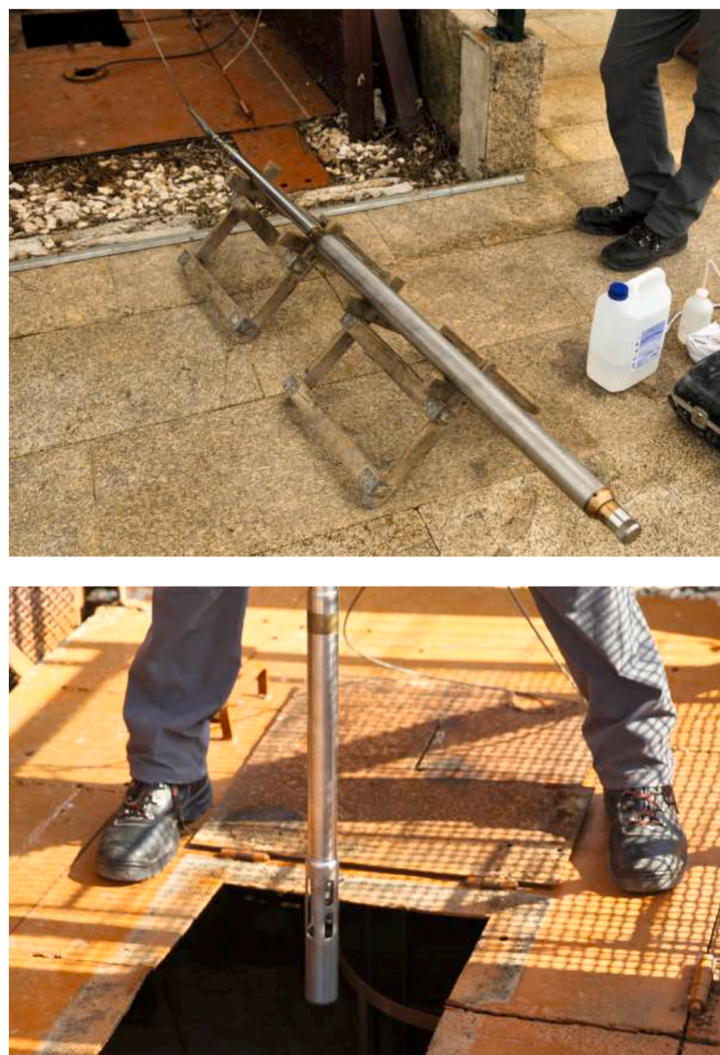
Fig. 1. Downhole probe for water sampling and on-site parameters (Barbara shaft, Urgeirica, Portugal).
