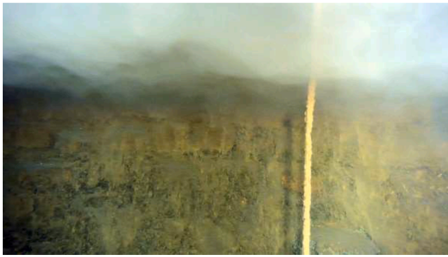
Fig. 4. Stratification in a flooded underground mine taken with a shaft camera. The camera is just slightly below the transition from a murky to clear water (courtesy: Thorsten Gökpinar; image optimized with colour and contrast enhancement, image width \approx 1 m).
