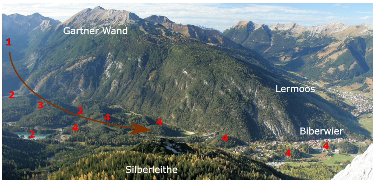
Figure 1.3: Overview of the Fernpass rockslide near Biberwier (in the left of the image). 1: rockslide source area, 2: Fernpass lakes, 3: northern branch of the rockslide with 4: selected Toma Hills. Direction of view to the south-west (photographer: Ch. Wolkersdorfer)
