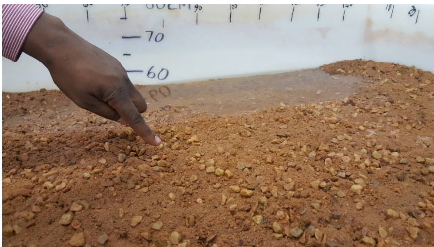
Figure 5.15: Development of lateral depression during experiment № 1. Spacing of the marks 10 cm (photographer: K.S. More)
