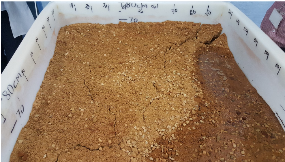
Figure 5.11: Beginning of the formation of cracks and a water-filled depression during experiment № 1. Spacing of the marks 10 cm (photographer: More KS)
