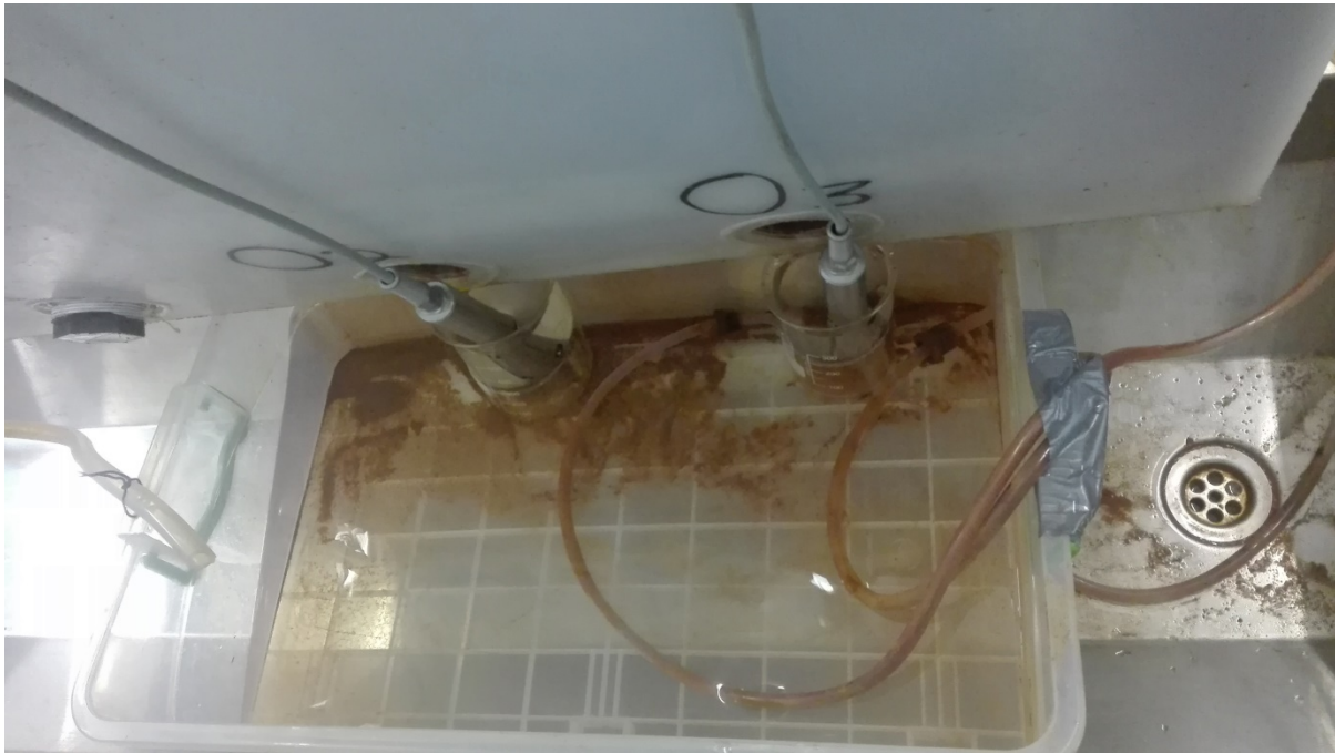
Figure 5.18: Tracer test setup during experiment № 5B, probes in the beakers placed adjacent to the outlets to measure the electrical conductivity
